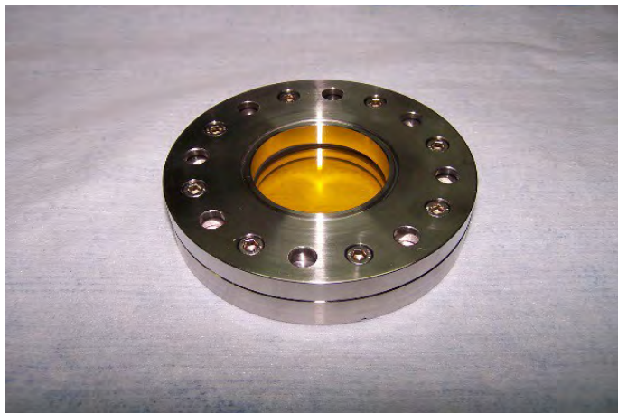
Ultra high vacuum flange fitted with an AR coated ZnSe disc.
