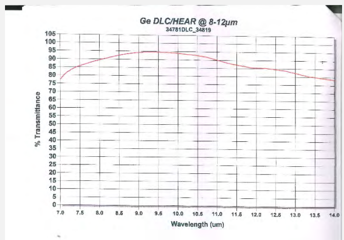
Germanium transmission curve AR/DLC coating:
